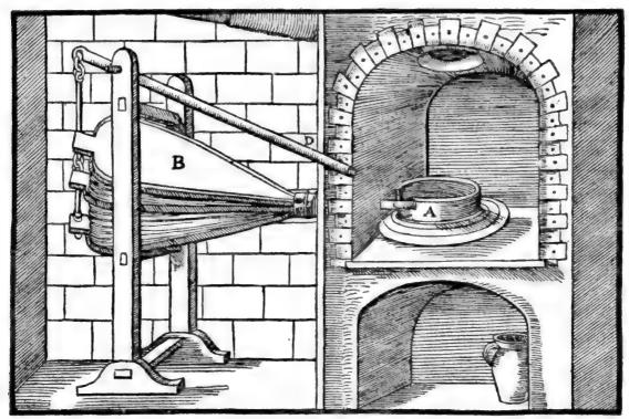
A-Iron Hoop. B-Double Bellows. C-Its nozzle. D-Lever.
